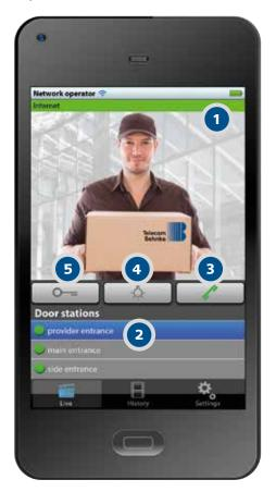
The bar • shows whether the video is received via LAN or 3G/4G. Colour and length of the bar indicate the quality of transmission. The names of the configured door telephones are shown in the list • at the bottom.
